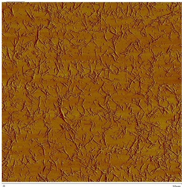
Figure 2. AFM micrograph of CNC obtained from microcrystalline cellulose. [Color figure can be viewed in the online issue, which is available at wileyonlinelibrary.com .]
